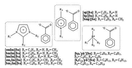
Fig. 2. List of benzoate based RTILs produced.
