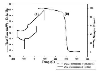
Fig. 3. (a) DSC thermogram of [ep][ba]; (b) TGA thermogram of [bmIm][ba].
